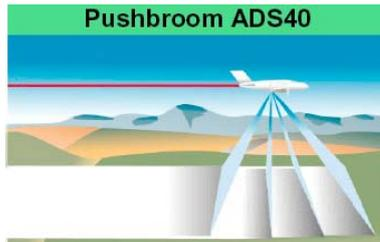
Figure 1. The pixel carpets produced by the Leica ADS40 camera.
