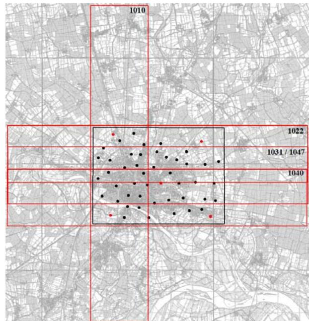
Figure 10. Outline of the 2000 m flying height block. The distribution of the control points is also shown; the black dots are used for DG assessment.
