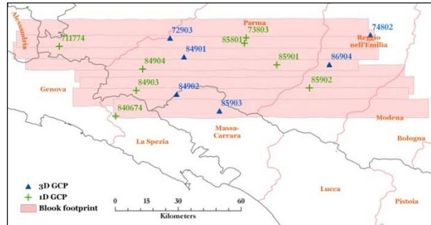
Figure 9. Outline of the *Emilia* block: the eight strips are shown, together with full CKPs (blue triangles) and pure altimetric ones (green crosses).
