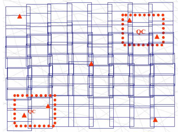
Figure 7.1 Calibration scheme suggested by Applanix
